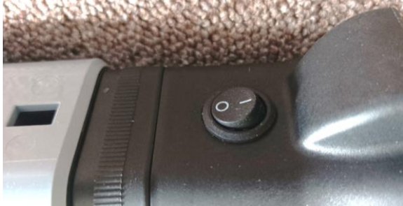
Representation of switch position OFF ("O")
