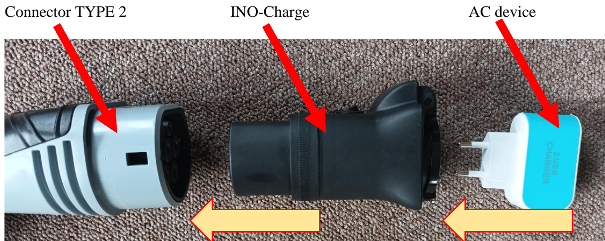
Representation of individual devices for their subsequent connection
